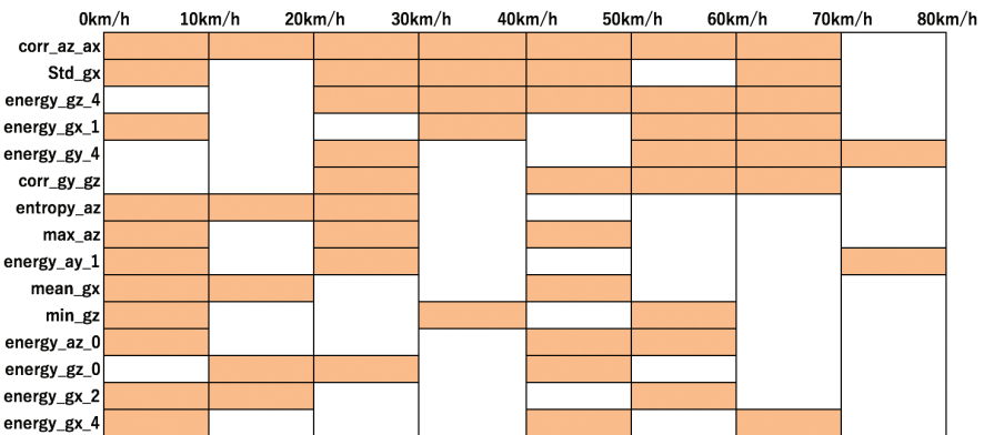
Fig. 10. Details of the selected features by using the SFFS in different speed ranges
