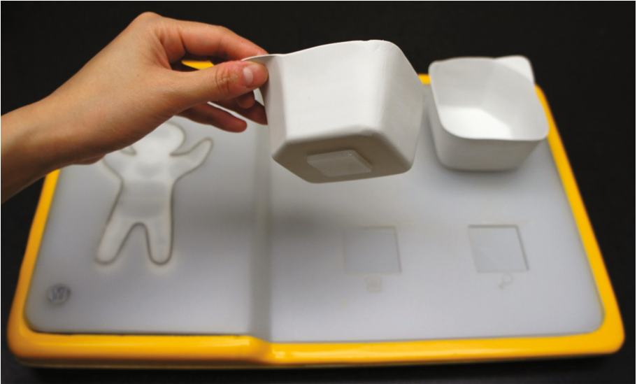
Fig. 3. Interactive board with “Cibo” character (left) and serving containers with flat bottom piece to facilitate contact with force sensors (right)
