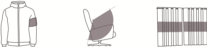
Fig. 8. Considered positions of the textile interfaces: proximal textiles (left), textiles in the extended surrounding area (middle), textiles in the surrounding space (right).
