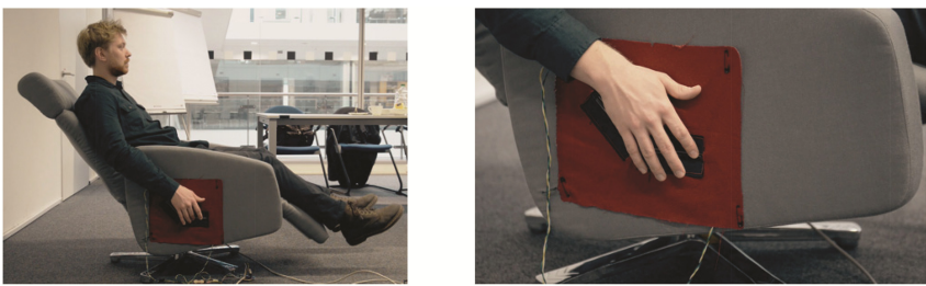
Fig. 2. Extended surrounding area demonstrator: motorized armchair with a textile interface.
