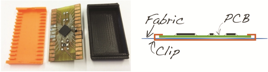
Fig. 6. The orange clip provides bins for the endings of the conductive thread. The PCB just has simple contact areas on the bottom side and is pressed against the fabric by the orange plastic clip. The black part is the top case of the enclosure. (Color figure online)
