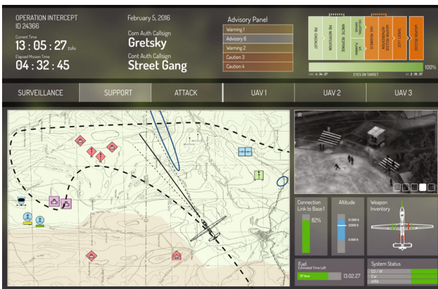
Fig. 3. Authority Pathway shared SA view integrated into an example overall mission SA display which also includes UAS sensor feed, maps, and other important mission information.
