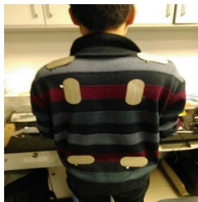
Fig. 1. The arrangement of force sensors
