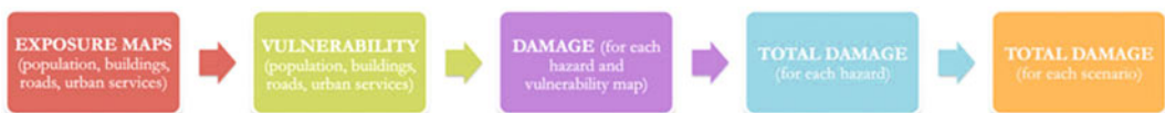
Fig. 6 Steps in the vulnerability analysis in the VOLCANDAM approach (after Scaini et al. 2014). See text for details
