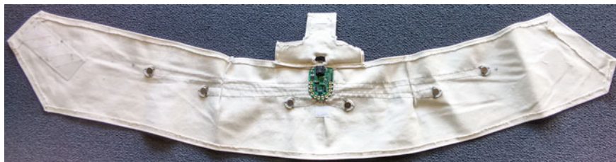
Fig. 10.2 Augmented belt embedded with six vibrating actuators (garment design and manufacturing by J. Berzowska and A. Bachmayer—XS Labs, Concordia University)
