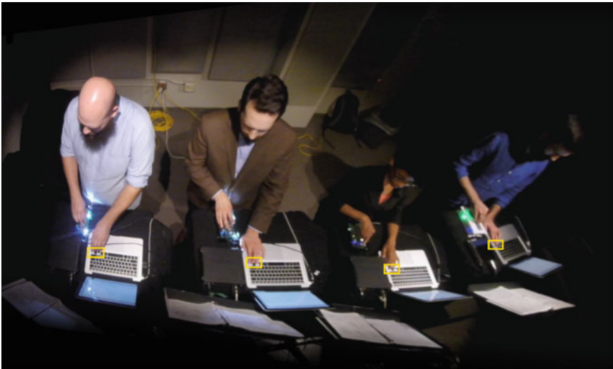
Fig. 9.8 For Of grating impermanence , the performers use their right hands to pluck a harp of virtual strings and their left hands to press the arrow keys on the laptop keyboard (see the yellow rectangles above). The right arrow advances to the next chord for the harp, and the left arrow goes back to the previous chord
