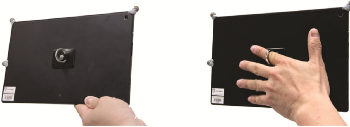
Fig. 4. Holding the MagicPad with one hand with the aid of the ring
