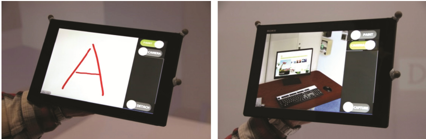
Fig. 5. Paint mode (left) and Camera mode (right) of the MagicPad HD
