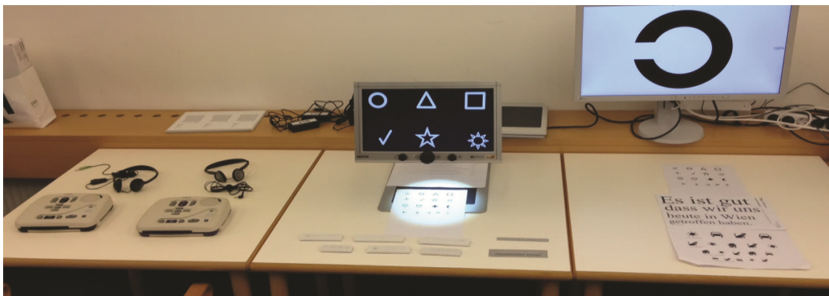
Fig. 1. Test setting for the evaluation of users’ physical condition. Hearing test, tactile perception test and visual perception test (from left to right).
