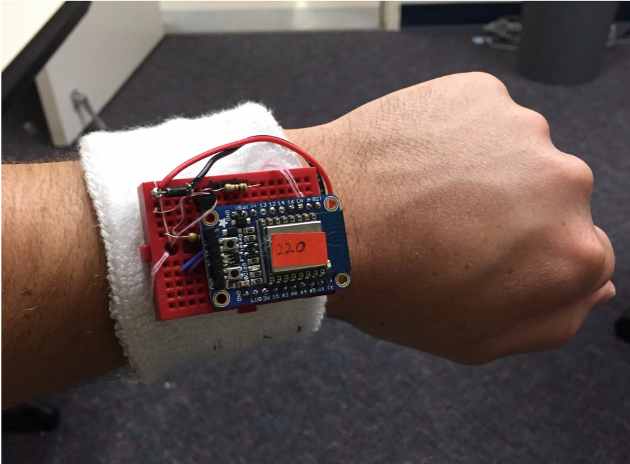
Fig. 3. Wristband for tool and object proximity detection via WiFi signal strength.
