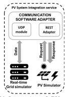
(b) Integration of PV and Real-Time grid simulators
