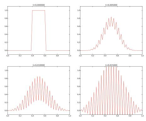
**Fig. 3.3** Forward Euler scheme for F = 0.51
