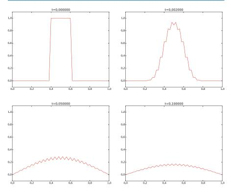
**Fig. 3.1** Forward Euler scheme for F = 0.5
