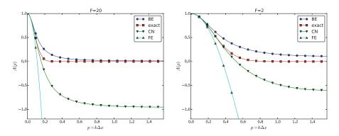
Fig. 3.9 Amplification factors for large time steps
