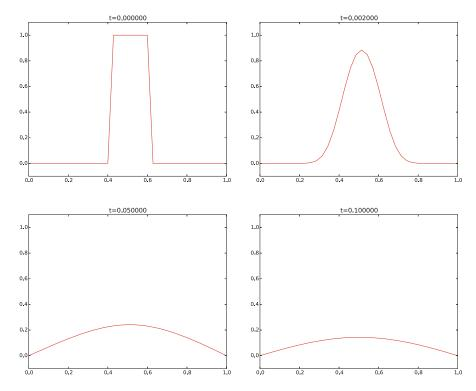
**Fig. 3.2** Forward Euler scheme for F = 0.25
