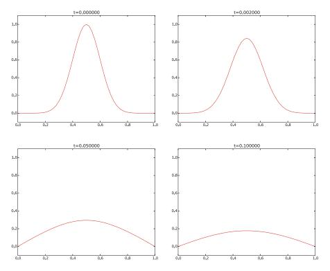
**Fig. 3.4** Forward Euler scheme for F = 0.5
