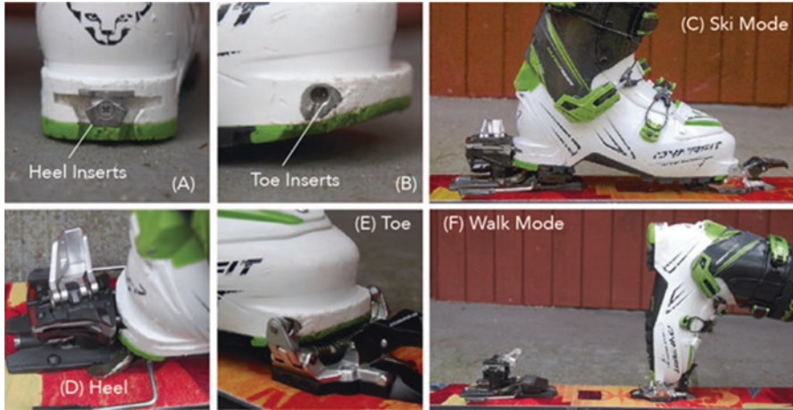
Fig. 2 (a) Heel inserts, (b) toe inserts molded into ski boots, (c) Tech/Pin binding-boot in ski model, with the toe and heel of the boot engaged, (d) heel of the boot engaged, (e) toe of the boot engaged, (f) walk mode with the heelpiece disengaged and only the toe piece of the binding engaged with the boot
