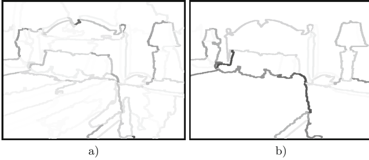
Fig. 3. Computation of b_{i,j} on a sample scene (i.e., the one in the sixth row of Fig. 5): (a) b_{i,j} values on the initial over-segmentation; (b) b_{i,j} values on the final result after all the merging steps. The boundary of the segments have been colored proportionally to the similarity between the two touching segments (black corresponds to low b_{i,j} values and white to large ones)
