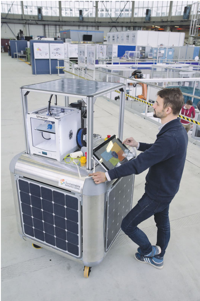
Fig. 6 CubeFactory: mobile, self-sufficient mini-factory
