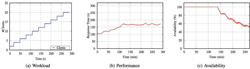
**Fig. 16.** Impact of workload on MapReduce performance and availability with #Nodes = 20, #MC = 10
