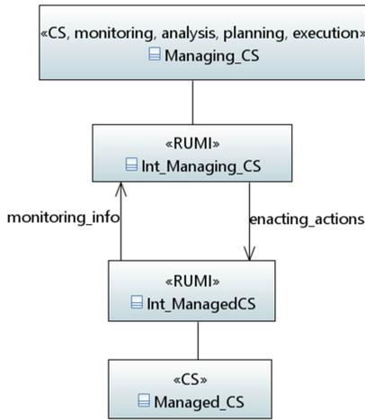
Fig. 2. Hierarchical control pattern
