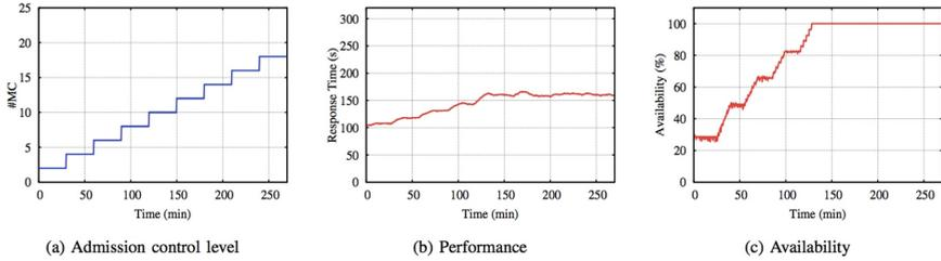
**Fig. 18.** Impact of admission control on MapReduce performance and availability with #Nodes = 20, #Clients = 10
