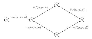
Fig. 2. Part of an FSM with controllability problems
