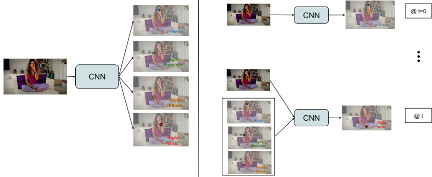
Fig. 1. A description of our model for the task of body pose estimation compared to pure feed forward nets. Left: Feed forward networks make independent predictions for all body parts simultaneously and fail to capture contextual cues for accurate predictions. Right: Body parts are predicted sequentially, given an image and all previously predicted parts. Here, we show the chain model for the prediction of Right Wrist , where predictions of all other joints in the sequence are used along with the image.
