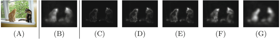
Fig. 3. Class saliency maps obtained from the VGG16-net fine-tuned with the PASCAL VOC 2012 dataset. (A) an input image, (B) average of [(E)–(G)], (C) conv1_1, (D) conv2_1, (E) conv3_2, (F) conv4_2, (G) conv5_2
