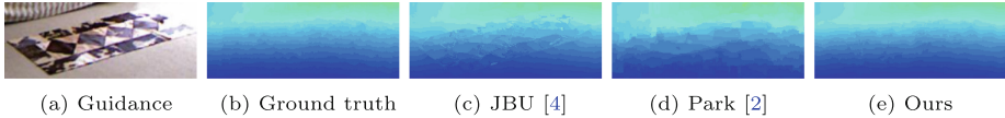
Fig. 11. Comparisons of different joint upsampling methods on the texture-copying issue (the area carpet on the floor contains unwanted texture structures).
