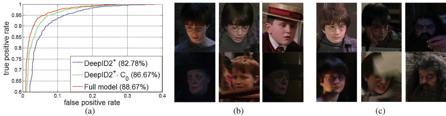
Fig. 8. (a): ROC of face verification on Accio-1 [30] dataset. The number in the legend indicates the verification accuracy. (b) and (c): negative and positive pairs failed to be matched by DeepID2+ [7] but successfully matched after adaptation by our approach.
