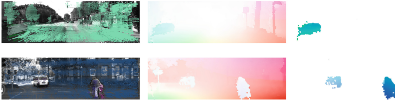
Fig. 4. A visualization of motion hypothesis (left), optical flow (middle), and scene motion flow (right). Camera motion is explicitly removed from scene motion flow. In the image of the cyclist we show that although multiple motion hypotheses are discovered by RANSAC (in two colors), a final smooth motion over this non-rigid entity is estimated with continuous optimization. (Color figure online)
