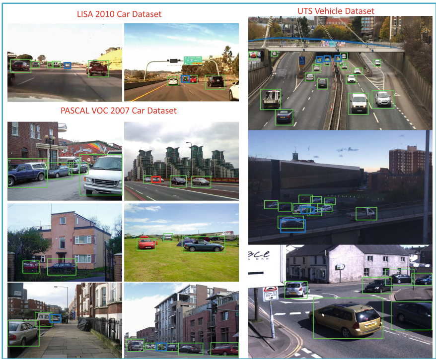
Fig. 6. Examples of successful and failure cases for detection (a green box denotes correct localization, a red box denotes false alarm and a blue box denotes missing detection) (Color figure online)
