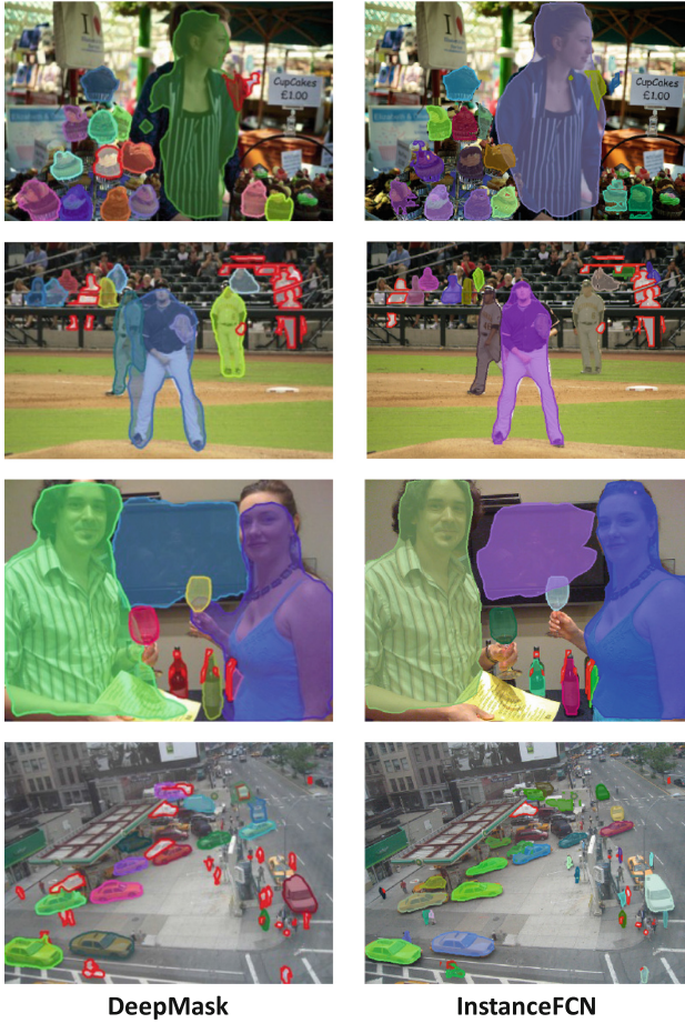
Fig. 8. Comparisons with DeepMask [8] on the MS COCO validation set. Left: DeepMask, taken from the paper of [8]. Proposals with highest IoU to the ground truth are displayed. The missed ground-truth objects (no proposals with IoU > 0.5 ) are marked by red outlines filled with white. Right: Our results displayed in the same way. (Color figure online)
