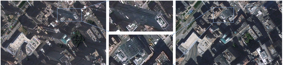
Fig. 2. Satellite context. A wide baseline is a necessity to reach reasonable depth accuracy, but brings severe occlusion problems. A facade side is typically visible only in one image (see closeups). Note also the high proportion of shadow and the time-varying objects as cars
