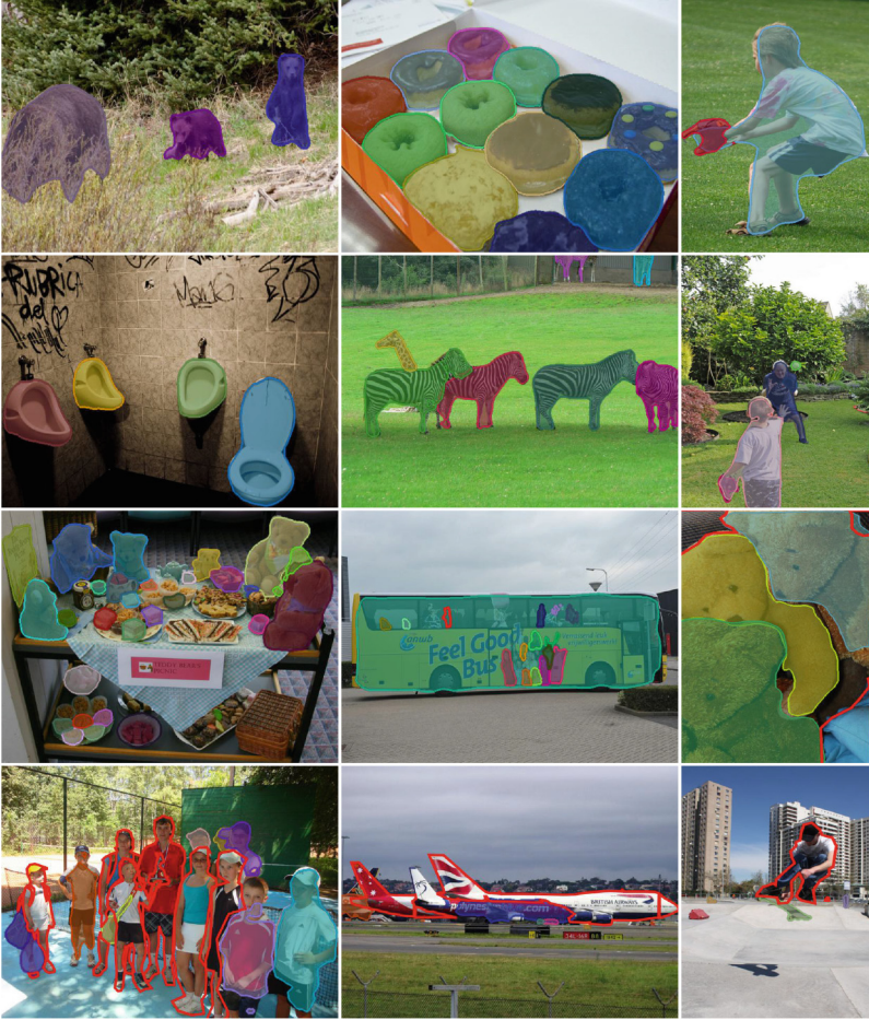
Fig. 4. SharpMask proposals with highest IoU to the ground truth on selected COCO images. Missed objects (no matching proposals with IoU >0.5) are marked in red. The last row shows a number of failure cases.
