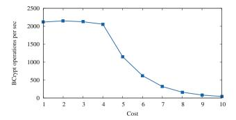
**Fig. 3.** Berypt performance as a function of the value of cost. Up to cost = 4, the single CPU can perform more than 2,000 operations per second.
