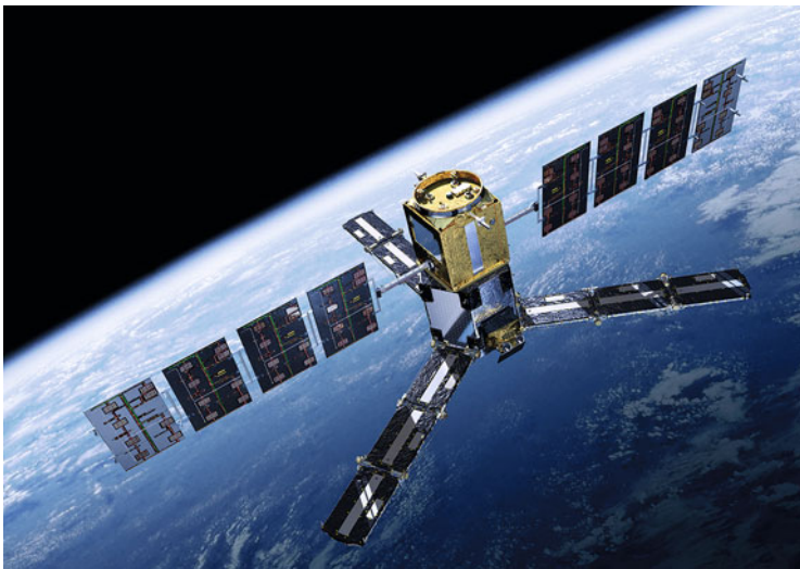
Fig. 17.6 Artist's conception of the SMOS satellite, a downward-looking interferometric array operating at 21-cm wavelength and imaging the Earth at a resolution of 35 km. The length of each of the three arms of the array is 4 m, and the array is tilted by 32^\circ to the tangent plane of the Earth below it. Image courtesy of and © European Space Agency.
