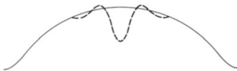
Fig. 11.2 Subtraction of the point-source response (broken line) at the maximum of a broad feature, as in the process CLEAN. Adapted from Clark (1982).
