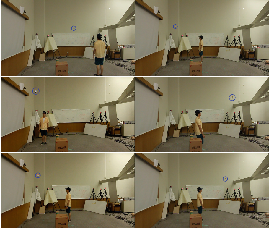
Fig. 6. Snapshots of quadrotor following the movement of a person
