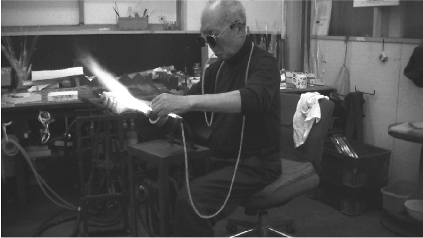
Fig. 2. Processing position of engineer with flame burner
