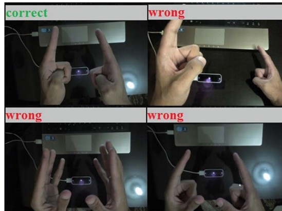
Fig. 2. Finger positions relative to the sensor
