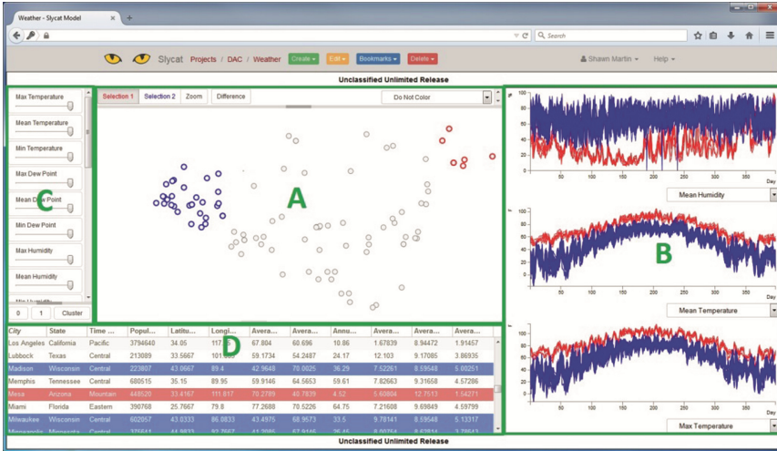
Fig. 4. Dial-a-Cluster interface divided into ROIs for the eye tracking analysis. A is the Cluster Pane, B is the Graph Pane, C is the Slider Pane, and D is the Metadata Pane.
