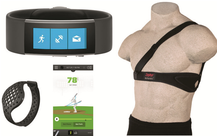
Fig. 4. Wearable sensing technologies: upper left is the Microsoft Band 2 [ http://www.microsoft.com/microsoft-band ]; lower left is the MOOV now activity bracelet that supports 3D motion tracking [ http://welcome.moov.cc/ ] and the Zepp Baseball sensor output [ http://www.zepp.com ]; right is Zephyr Technologies' BioHarness 3 wearable sensor [ http://www.zephyranywhere.com/ ].
