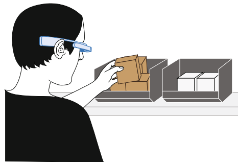
Fig. 3. Pick-by-Vision: Smart glasses provide order information in the pickers field of vision
