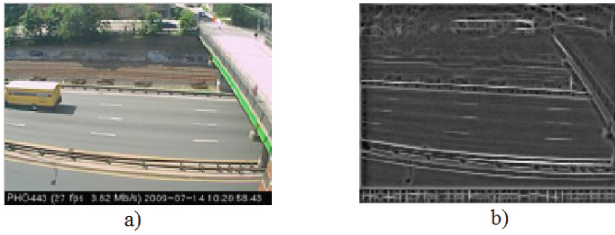
Fig. 5. Background modeling. (a) StreetLight frame t = 100 . (b) SY_1(x, y, t) .
