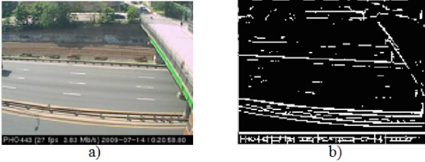
Fig. 6. Edge detection with PGSeg. (a) StreetLight , frame t = 100 . (b) I_s(x, y, t) .
