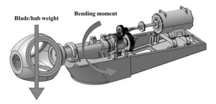
Fig. 9.4 Non-torque loadings and their effects on a typical 3-point suspension drivetrain
