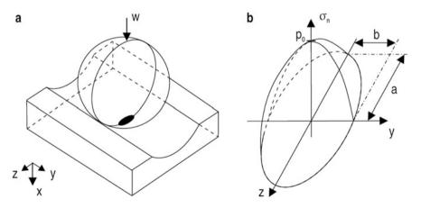
**Fig. 9.2** (a) Elliptical contact area in *black* and in (b) the corresponding surface stress distribution (Jacobs 2014)
