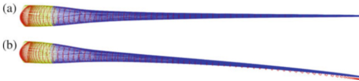
Fig. 18.16 DTU 10 MW RWT modal analysis initial deformation ( blue-yellow ), superposed to the blade geometry reference ( red ) at rated speed . (a) Straight blade. (b) Prebent-precone blade
