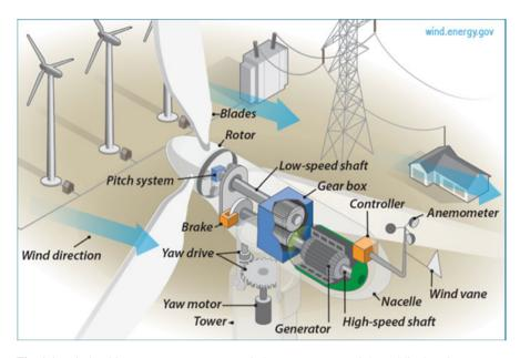
Fig. 1.1 Wind turbine components. Source: wind.energy.gov; copyright: public domain
