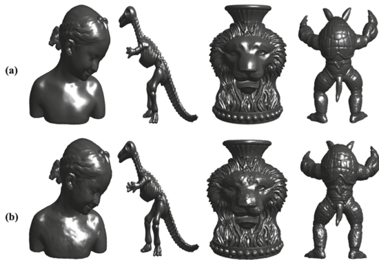
Fig. 4. Some models from the LIRIS Masking Database and their distorted versions: (a) reference meshes. (b) distorted meshes with noise addition.
