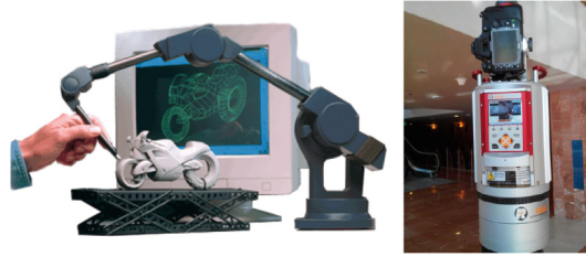
Fig. 1. 3D scanning devices. Left: A contact-based MicroScribe device (photo taken from [3]). Right: The Riegl VZ-400 terrestrial laser scanner.
