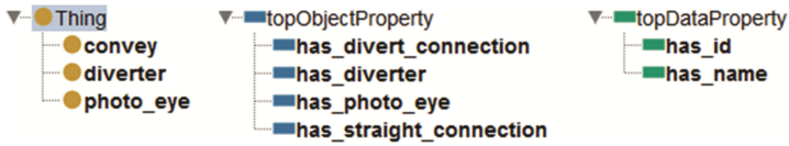
Fig. 2. BHS ontology consisting of Classes (left), Object Properties (Center) and Data Properties (Right) shown in Protégé.
