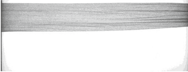
Fig. 4. A sample of sausage skin folding rejected by the LabView system, however manual inspection identified it as accepted, thus it a false positive case.
