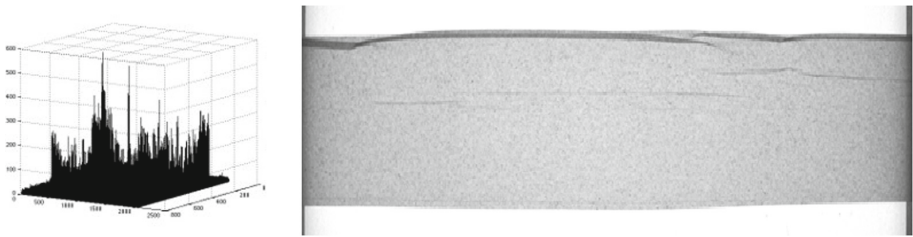
Fig. 6. Results of group 1. Showing a false positive defect. This image was found defective by LabView but shown correctly by our solution as non-defective. (left) Merit function values, (right) Actual image
