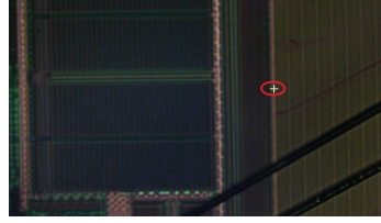
Fig. 4. The right position in EEPROM for laser fault attack (Color figure online)
