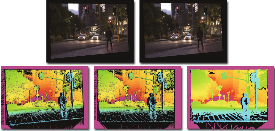
Fig. 3. Top: A rectified image pair \hat{I}_b and \hat{I}_m . Bottom, left to right: The resulting disparity map \hat{d} , the inversely transformed disparity map d , and the joint, bilaterally filtered result.
