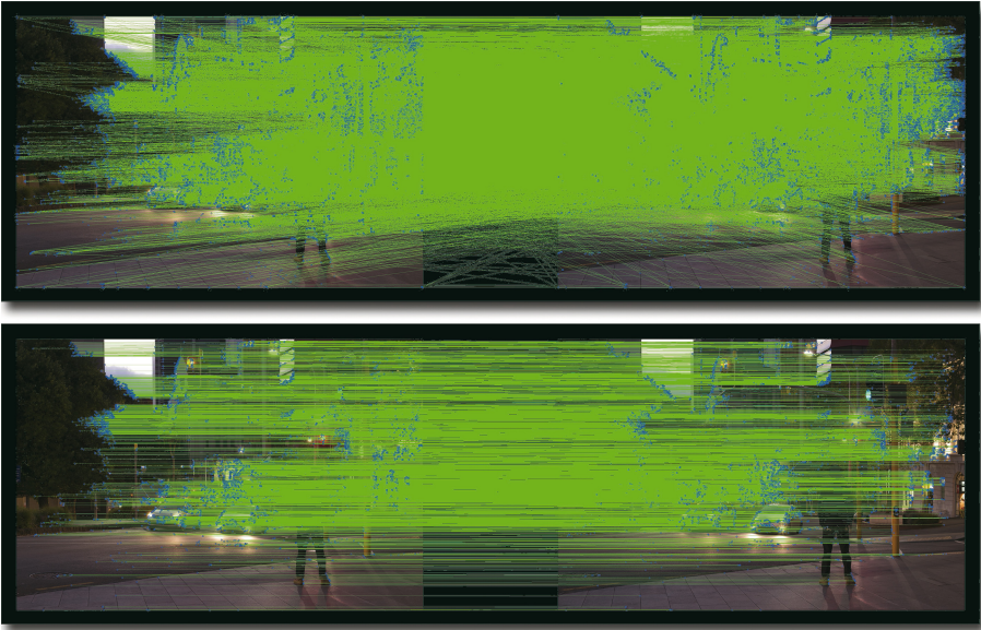
Fig. 2. Matched feature points before and after applying our filter
