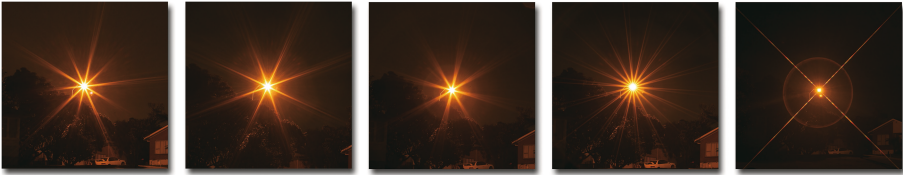
Fig. 1. Relationship between aperture shape and star effect. From left to right: Five straight blades aperture, eight straight blades aperture, eight curved blades aperture, nine curved blades aperture, and a circular aperture with a star filter
