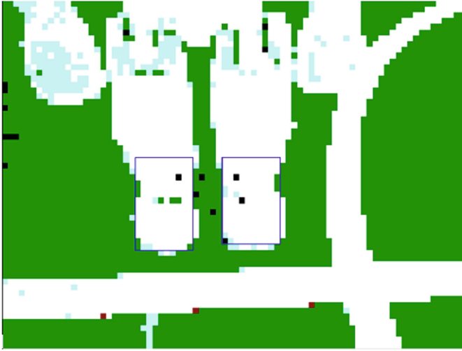
Fig. 4. The colour saliency provided from offnao (our offline debugger) with the feet bounding boxes shown in blue. The image also includes a difficult case of field line intersection which has not been classified as feet (Color figure online).
