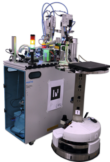
Fig. 2. Carologistics robotino approaching a ring station MPS.
