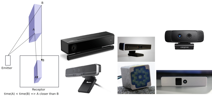
Fig. 3. The principle behind ToF sensors (left) and several sensors (from top left to bottom right): Microsoft Kinect 2, DepthSense, Creative Senz3D, Intel RealSense F200, Fotonic, PMD CamBoard pico ® .
