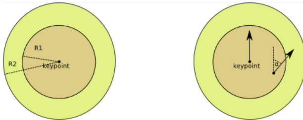
Fig. 8. Left: circular regions considered. Right: angle between the normal at a point in the R_1 region and the normal at the keypoint.
