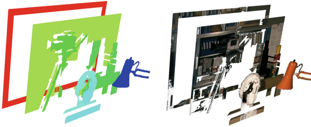
Fig. 1. Illustration of the rationale behind the algorithm. The left figure shows the coloured disparity levels of the dataset [25], while the right one depicts the original pixel colours. The algorithm is based on the observation that the objects share the similar disparity, as well as similar colour. This can be clearly seen on the red lamp in the foreground or the white statue on the left (Color figure online).
