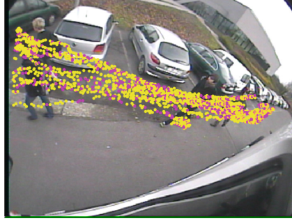
Fig. 8. Performance of both pedestrian detectors in function of the position in the image. Colored dots indicate which pedestrian detector performed best. Yellow: DPM. Magenta: FPDW (Color figure online).
