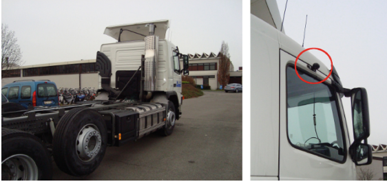
Fig. 12. Our test truck with the mounted commercial blind spot camera (circled in red) (Color figure online).
