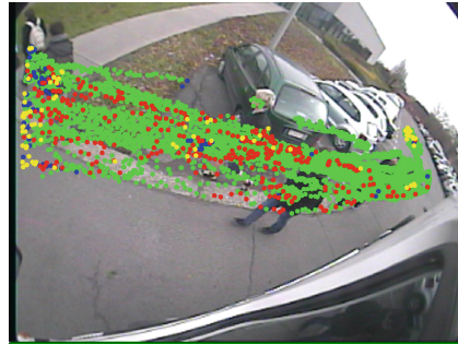
Fig. 9. Performance of the two transformation models in function of the position. Colored dots indicate which model performed the detection. Red: perspective model. Blue: similarity model. Green: both models. Yellow indicates missed detections (Color figure online).
